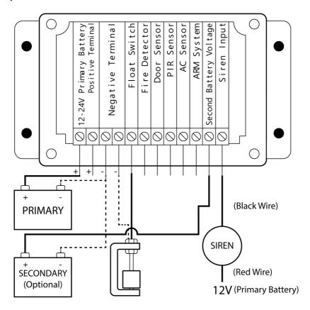
Wired sensors may require supply as well and are wired similar to the float switch.
