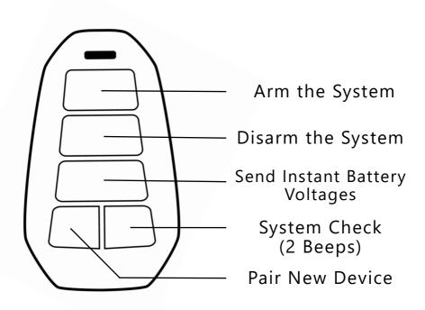
With the system armed, the system will send notifications via E-Mail and SMS (if configured) if the PIR or Door sensors detect movement
