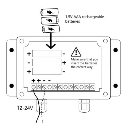
The device should beep once, twice then three times after power up. The IoT module is then ready to be used.
